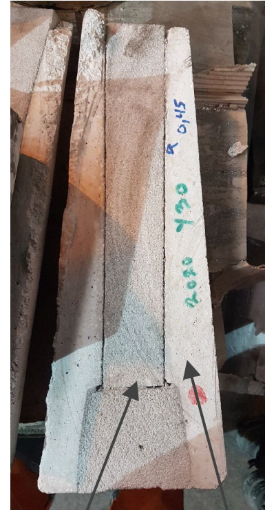
Photography of porous pug cut in middle plane
